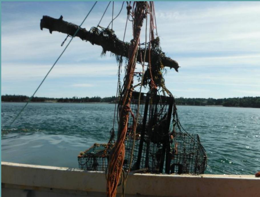
Photo 1. Traps being hoisted up alongside a vessel by a grapple during at-sea retrieval efforts in Saint Andrews, NB. Photo credit: Fundy North Fishermen's Association.
